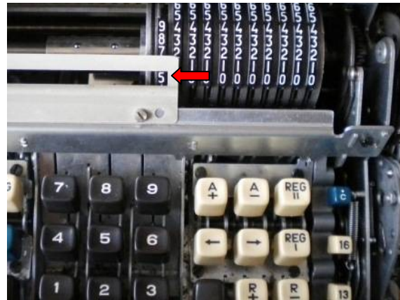
Key released, setting rotor steps left
