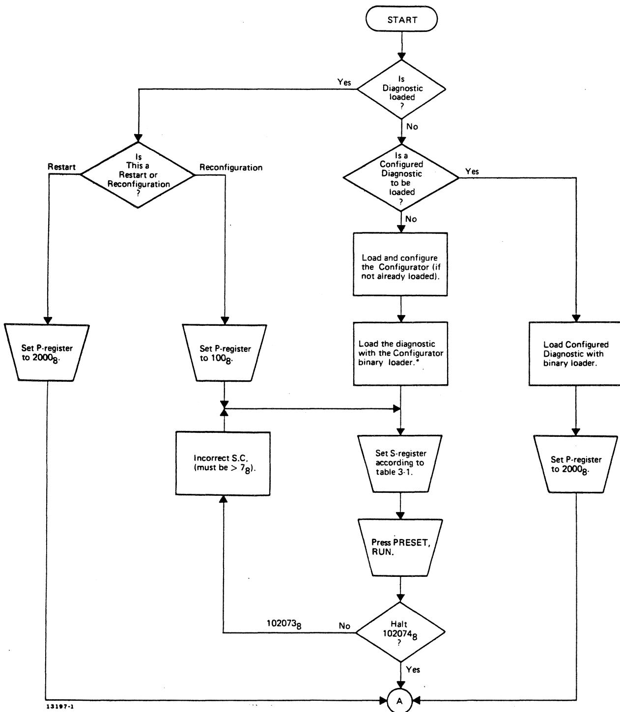
Figure 3-1. TST00-TST24 Operating Procedure Flowchart (Sheet 1 of 2)
