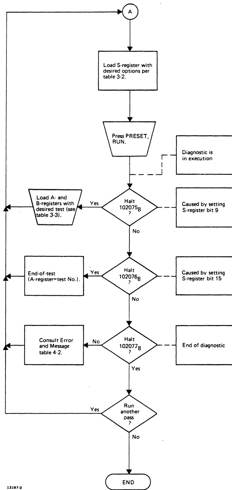
Figure 3-1. TST00-TST24 Operating Procedure Flowchart (Sheet 2 of 2)
