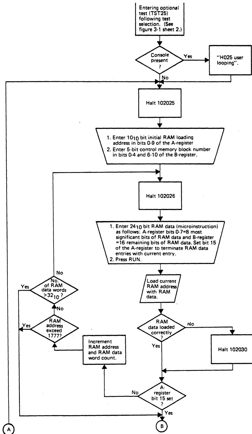
Figure 3-2. TST25 Operating Procedure Flowchart (Sheet 1 of 2)
