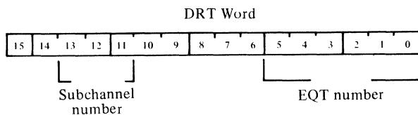
Each one-word entry in the DRT contains the EQT entry number of the device assigned to the logical unit, and the subchannel number within the EQT entry. The functions of logical units 1 through 6 are predefined in the RTE-C System as:
