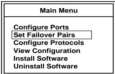
2 Add a Failover Pair by pressing **INS**. The program automatically assigns a default pair name. If previous pairs
