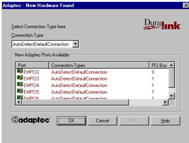
**1** From the **Adaptec New Hardware Found** dialog box, select the port to configure from the New AdaptecPorts Available list box.
