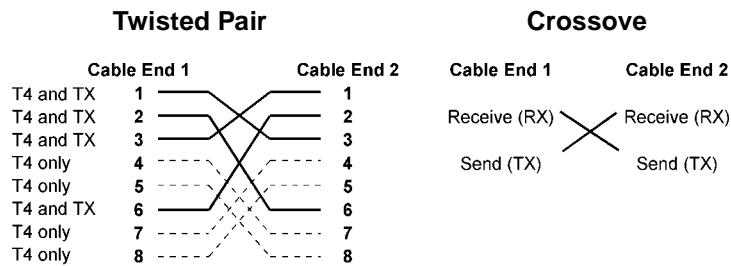
A simple network can be made by connecting a Quartet server directly to four workstations via crossover cables.
