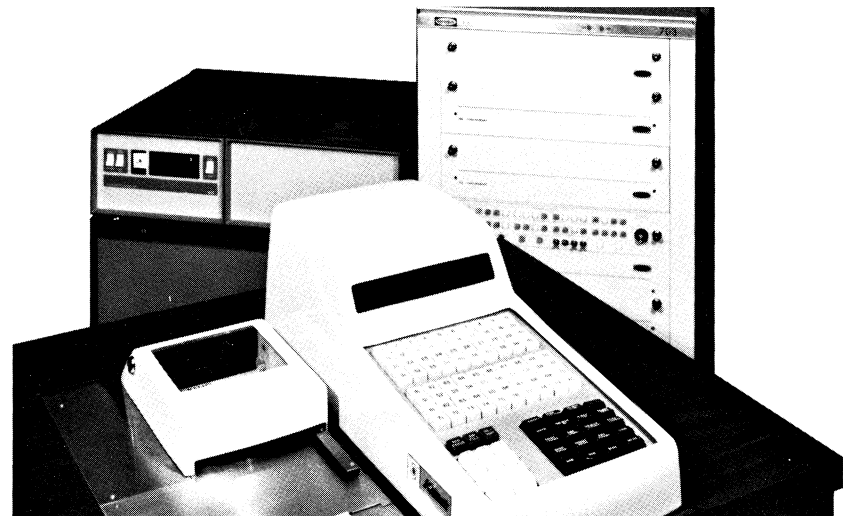
Ticket-writer terminal, disc memory and 703 computer are main elements in Kenotronic system.
