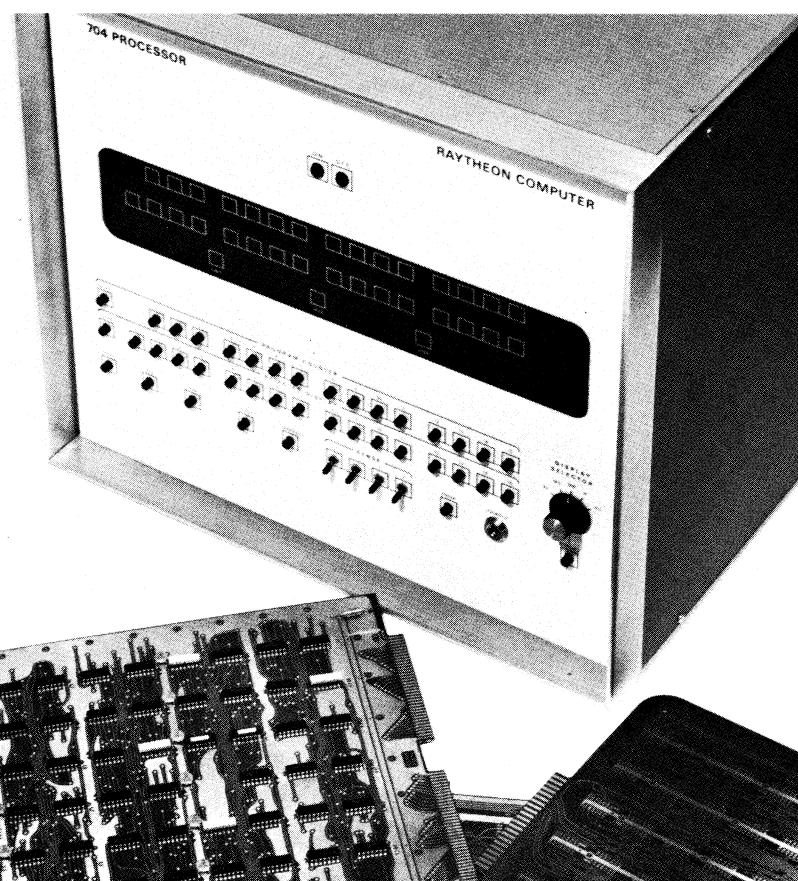
704 IC cards hold all logic and memory. User can choose optional utility cards with mounted IC sockets for special requirements.
