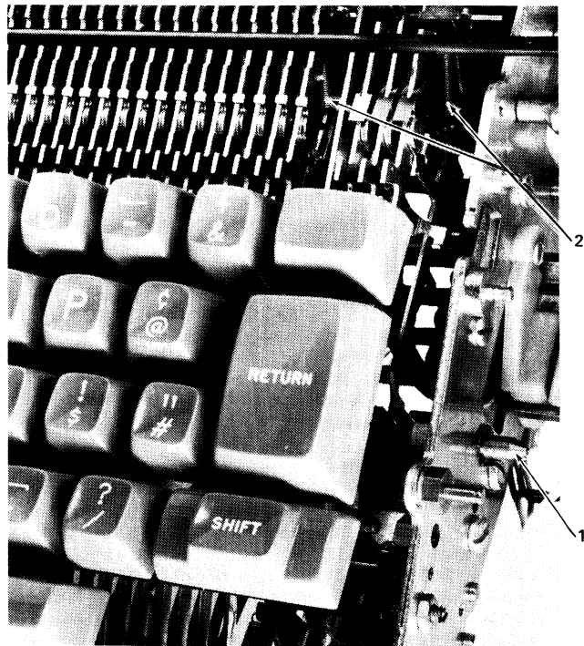
Figure 4-52. Keylever Interposer Removal (Top, Right View of Keyboard)
