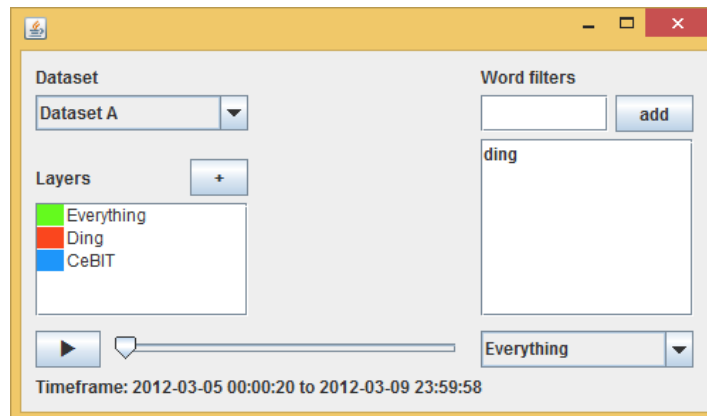
Figure 4.3: Screenshot of the desktop control application. It allows to edit different layers on the left side. On the right side, the textual filters can be modified. The slider at the bottom allows to filter temporally.
