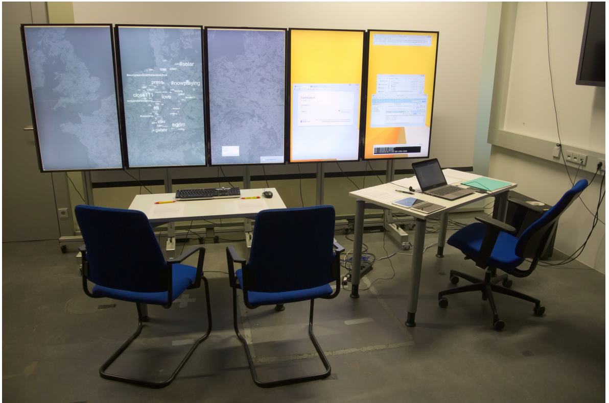
Figure 5.1: The setup for our user study. The three left-most screens are used for the map application. The fourth monitor allows the user to answer questions during the study, the right-most screen is used for diagnostic purposes only. At the left table, the users take place and operate the system.
