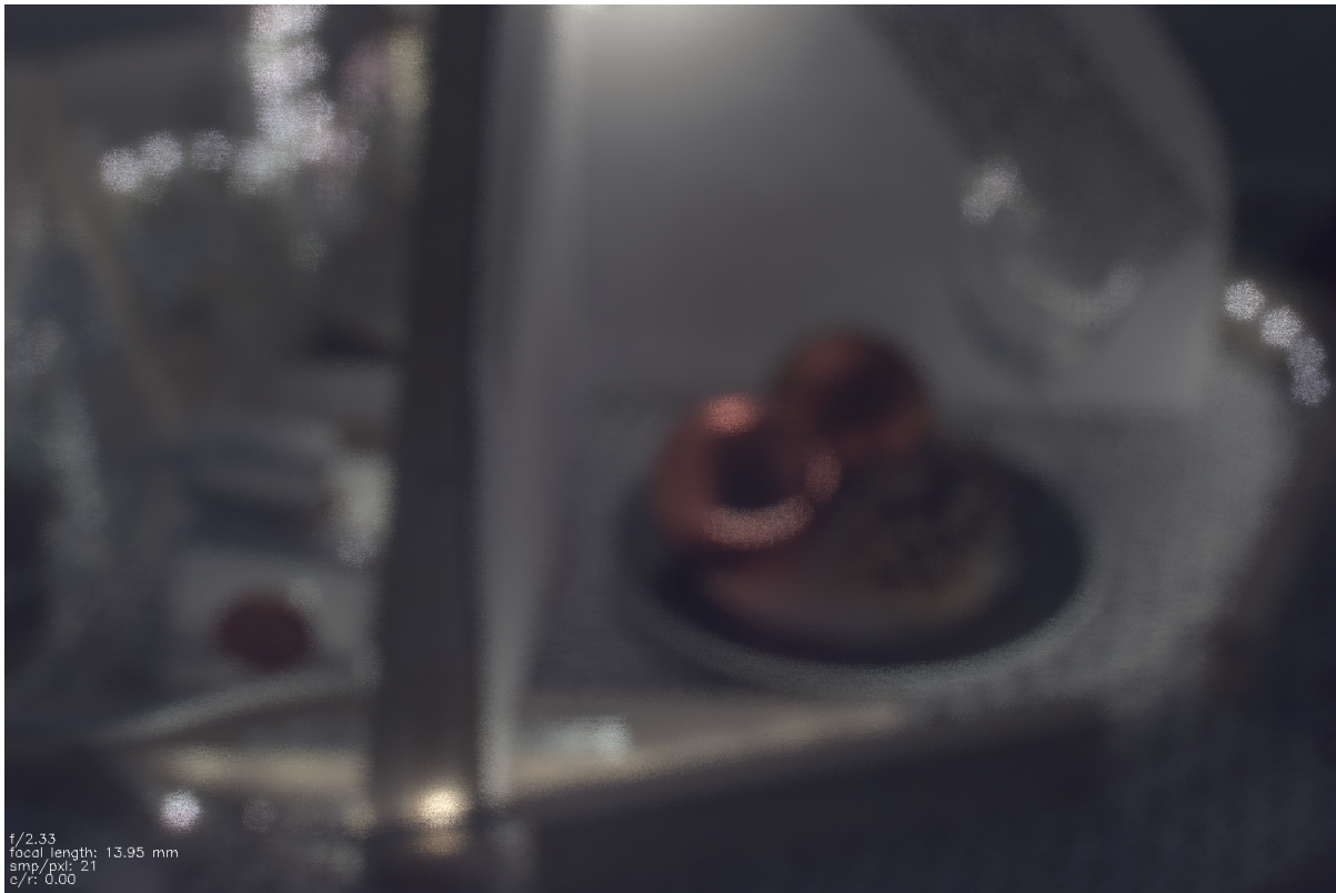
Figure 5.8: In this frame, raytracing was used to sample the sparsely rebinned light field. To acquire strong depth of field, the focus distance was chosen as 20 cm. 21 ray samples were taken per pixel. Distributed raytracing noise becomes visible. Note however, that bokeh effects are not cut off as it can be observed in Figure 5.4, missing data is interpolated.
