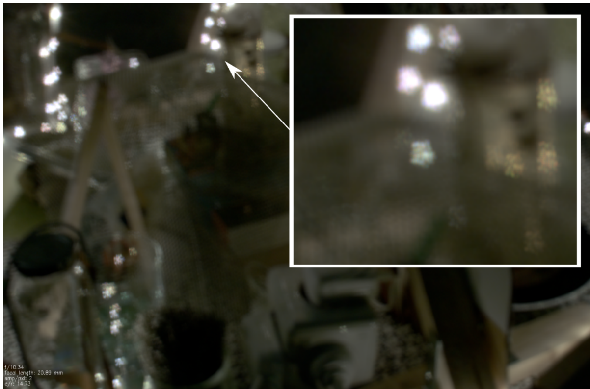
Figure 5.2: Frame from the bokeh movement. With the provided light field, bokeh effects are obtainable by selecting low focus distance and large aperture settings. Also note how the approach described in Section 4.3.3 enables shaped bokeh effects, in this case a pentagon.
