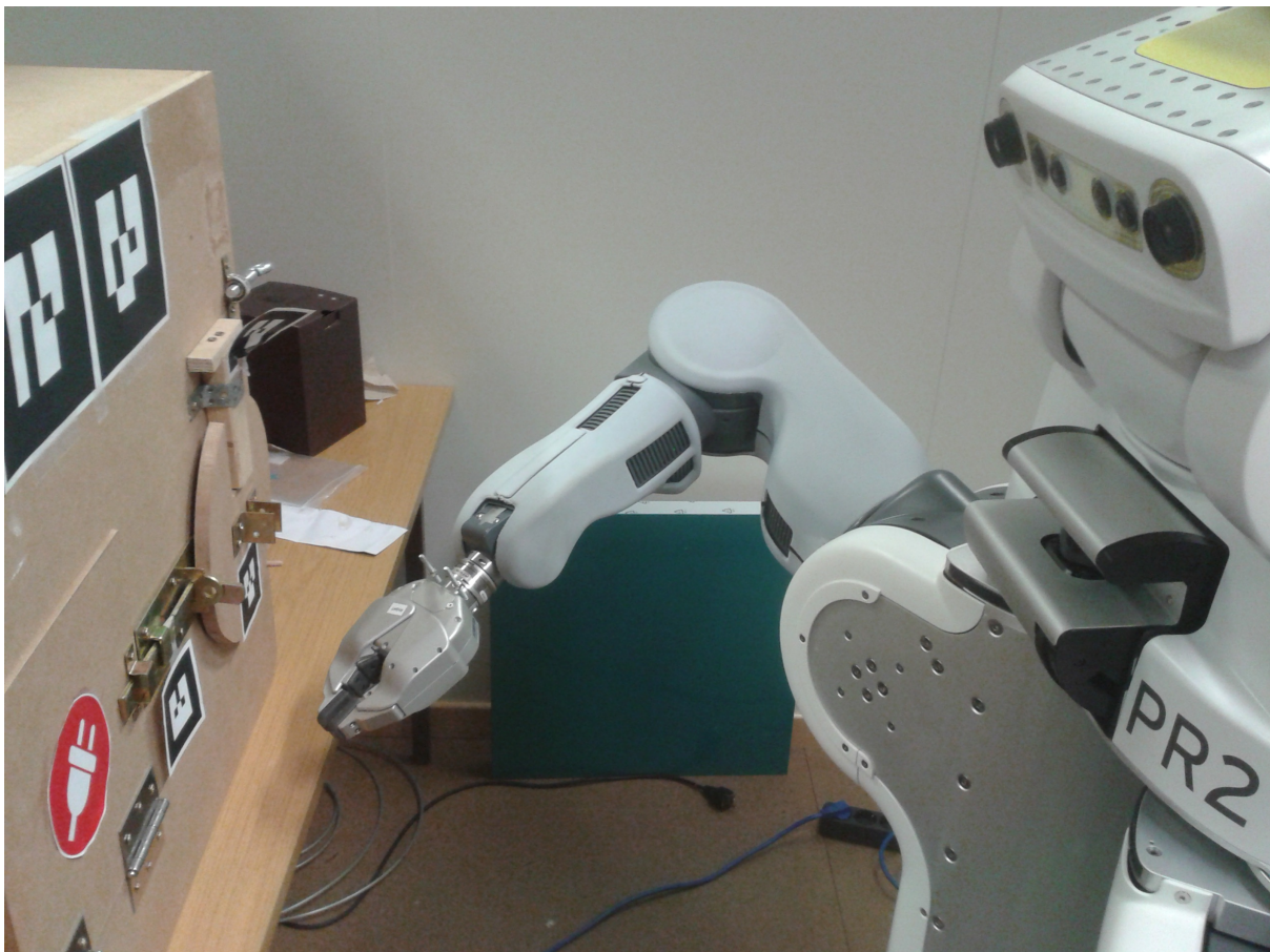
Figure 5.1: The robot in a joint state which prohibits further movement.
