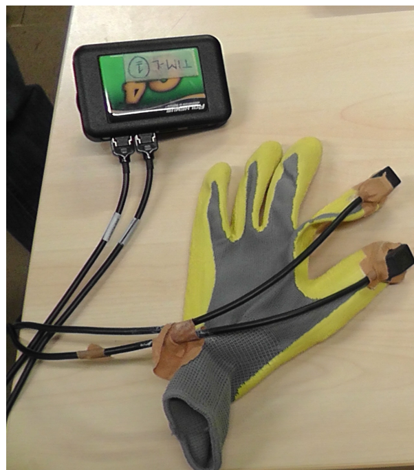
Figure 3.1: The left glove with the Polhemus G4 position tracking system attached to it.
