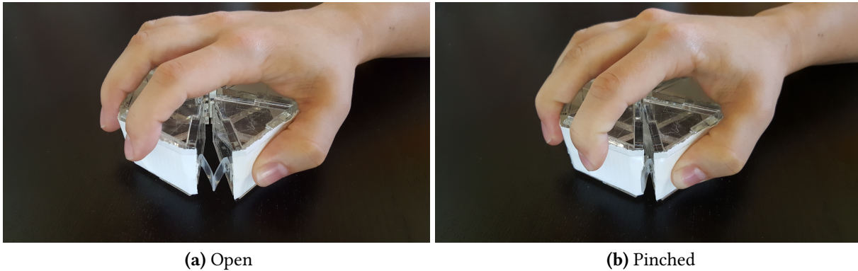
Figure 4.3: Pinch Dial – Values are selected through rotational input. Without force, the dial is in an open state (a) and through pinching (b) certainty can be expressed.
