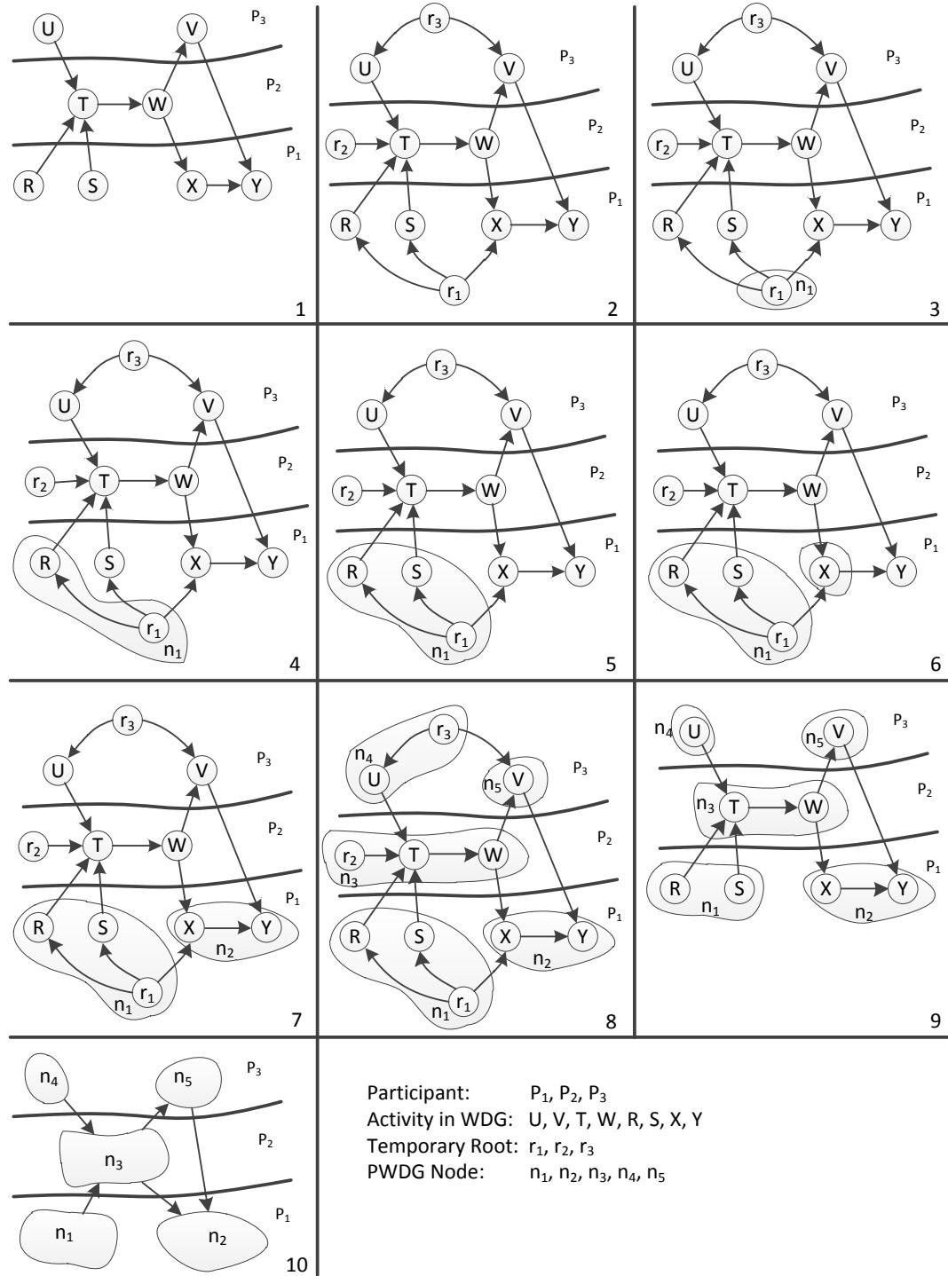
**Figure 5.4:** Construction of a PWDG (10) from a WDG (1) derives from [Kha08, Fig:41]
