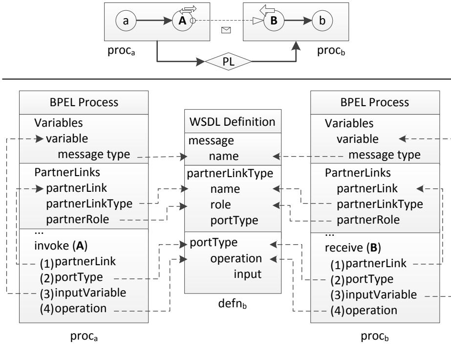
**Figure 3.4:** Conceptual Inter-Communication (top) and References in Processes (bottom)
