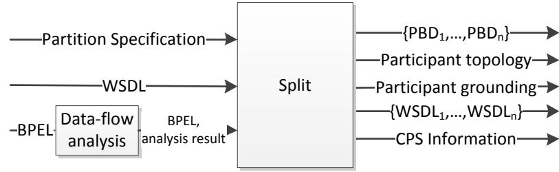
**Figure 1.1:** In- and Output of Splitting, the *Input* includes (1) partition specification, (2) BPEL, (3) WSDL, (4) and data-flow analysis result , the *Output* includes (1) a Participant Behavior Description (PBD) per fragment, (2) Participant Topology, (3) Participant Grounding, (4) a WSDL definition per fragment and (5) Cross-Partner-Scope (CPS) information .
