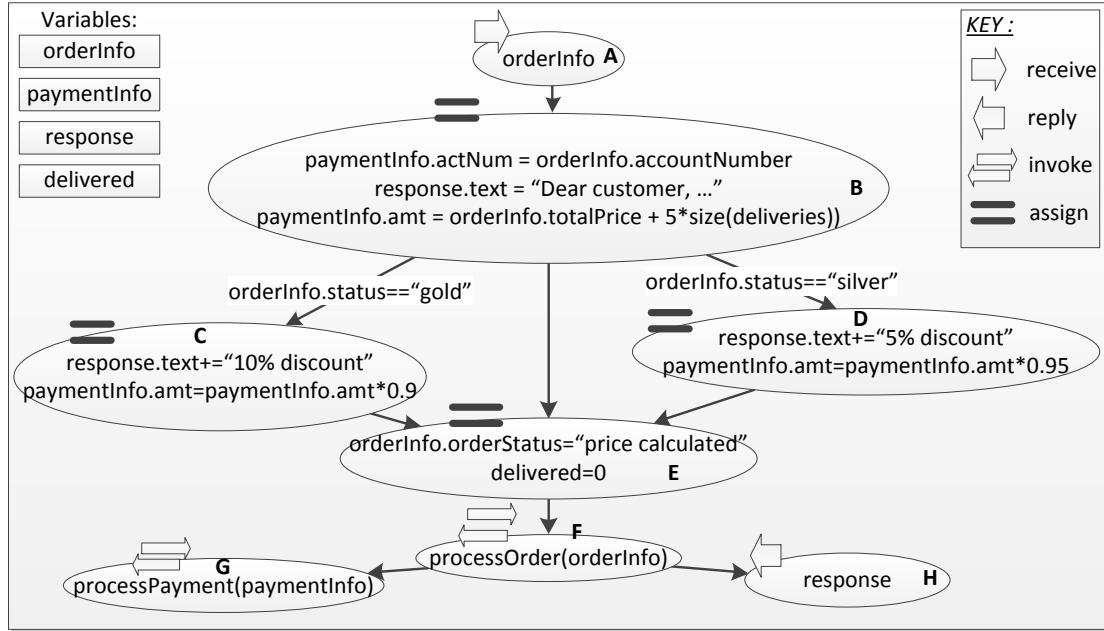
**Figure 3.2:** Ordering process that provides discounts to Gold and Silver customers [KKL08a, Fig. 1]
