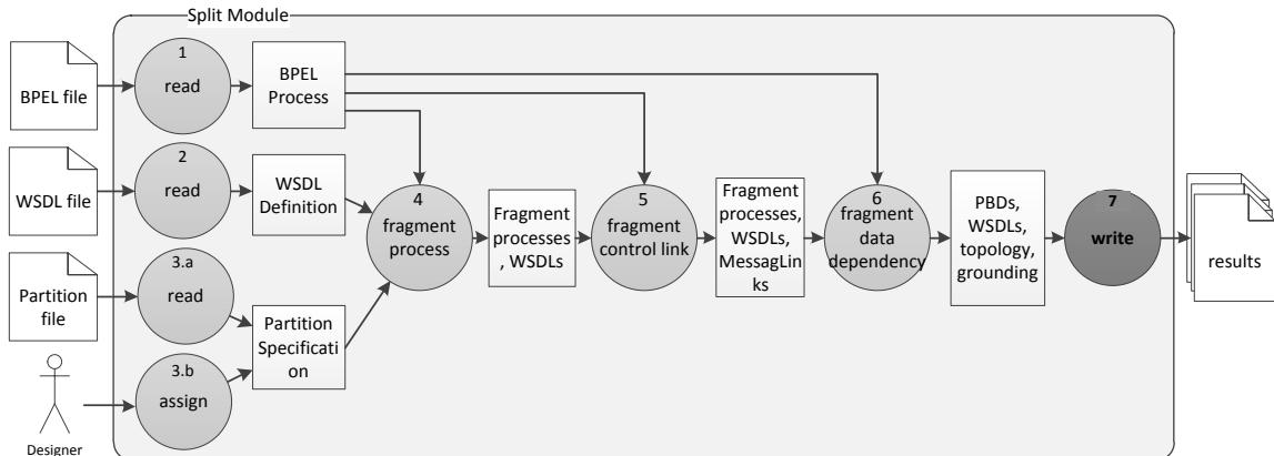
**Figure 6.1:** The Overview of the Split Module with Output in BPEL4Chor (Step 7) emphasized
