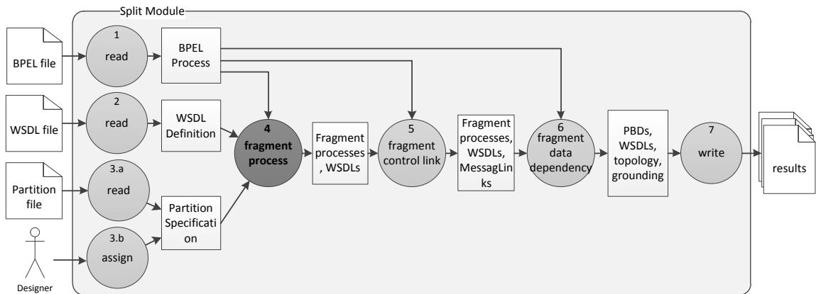
**Figure 3.1:** The Overview of the Split Module with Process Fragmentation (step 4) emphasized
