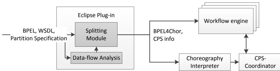
**Figure 1.2:** Architecture of the Process Fragmentation, the consumer of the output is workflow engines, Choreography Interpreter and CPS-Coordinator [Bor10, Abbildung 4.2].
