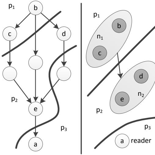
**Figure 5.5:** Example PWDG Illustrating Scenario for Creating Prerequisites, continued with Figure 5.3. Left: main process with partition  $P3 = \{p_1, p_2, p_3\}$  and the dependent writers  $A_d(a, x) = \{b, c, d, e\}$ , Right:  $PWDG_{a,x,P3} = (\{n_1, n_2\}, \{(n_1, n_2)\})$
