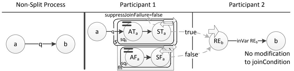
**Figure 4.3:** Splitting Control Link Concept with Variable Initialization
