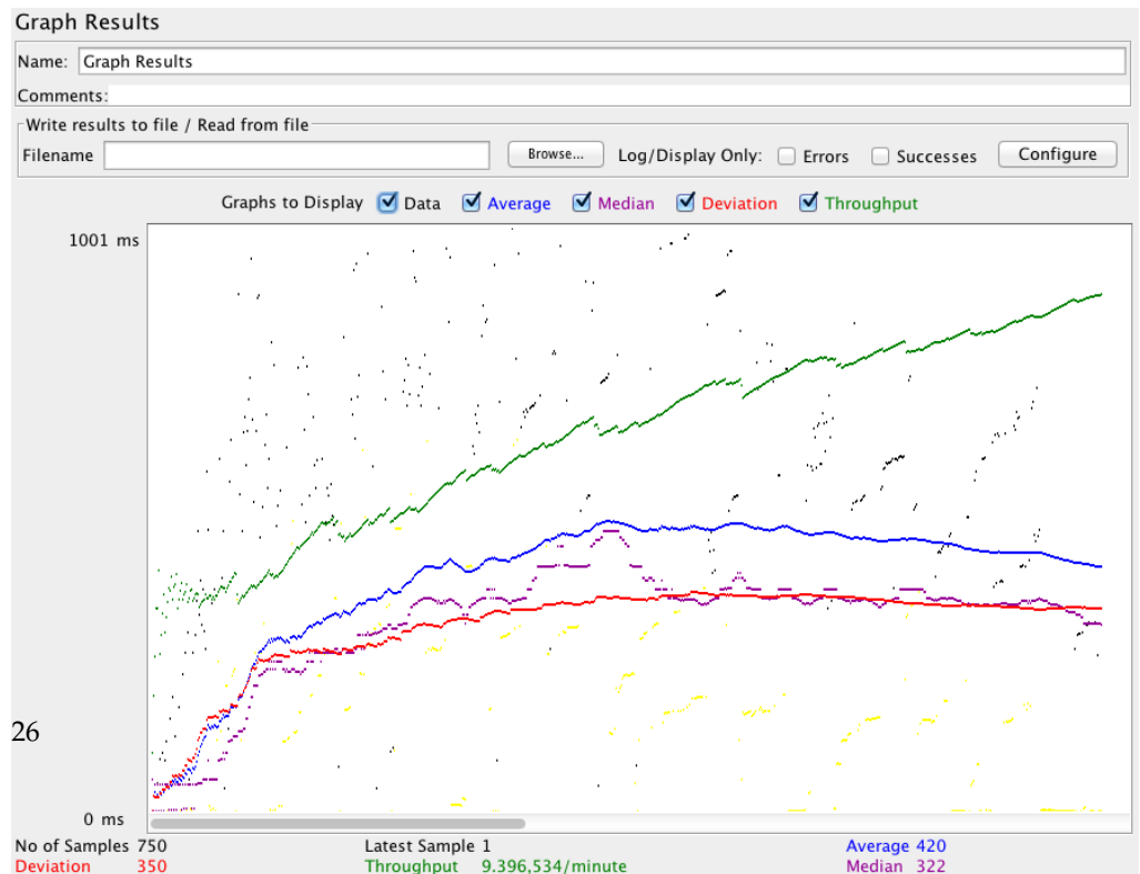
Figure 6.15. Graphical results of a test plan for the phpMyAdmin main screen web site with following properties: number of threads: 125, ramp-up period: 2, loop count: 3.
