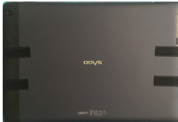
Figure 3.3: Velcro stripes used to always ensure the same grip
