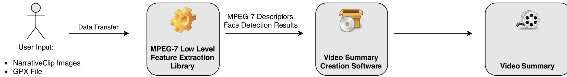
Figure 5.1: An overview of the context of our video summary creation system. Captured images are first transferred to the MPEG-7 extractor. MPEG-7 descriptors are then passed to our software that creates the video summary.
