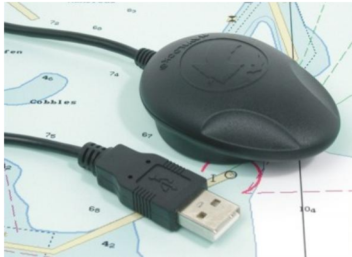
Figure 3.4: GPS receiver Navilock ul-402 for GPS data collection
