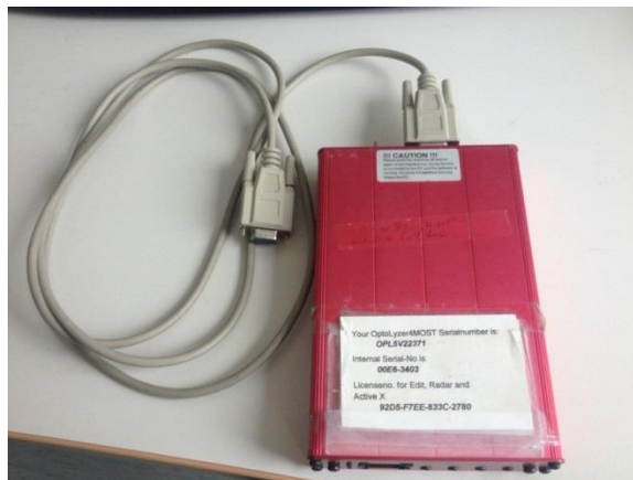
Figure 3.2: Optolyzer for MOST message detection
