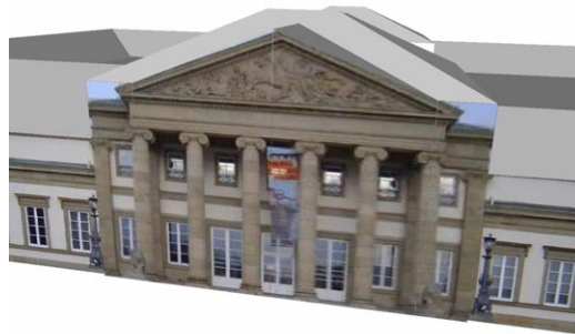
Figure 3. Resulting 3D building model with the extracted textures placed on the façade polygons.
