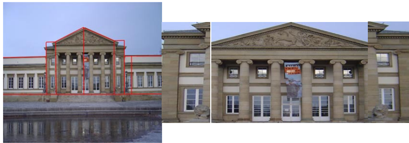
Figure 2. Projected 3D building model overlaid on the input photograph (left) and the extracted facade textures (right).
