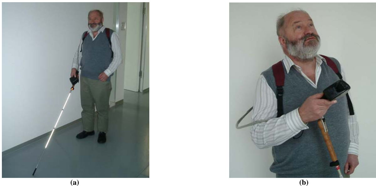
Figure 1: Our blind colleague during the first hardware usability test of the new navigation assistant. The sensor module can be clicked to the cane and can be handled with one hand (a). The system allows the identification objects by pointing at them using the sensor module (b) or can inform the blind user about the present location and distribute navigation advices by walking in corresponding navigation areas.
