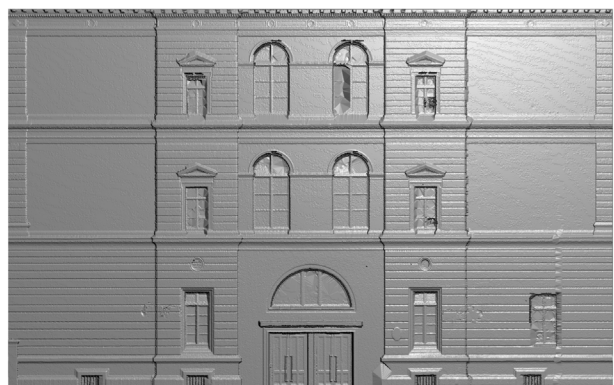
Figure 3. 3D Rendering of a single LASERMAP as a normal map.
