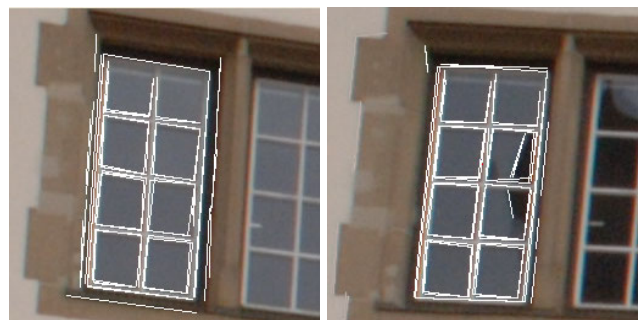
Figure 10. Selected 2D edges for an exemplary window in both images.
