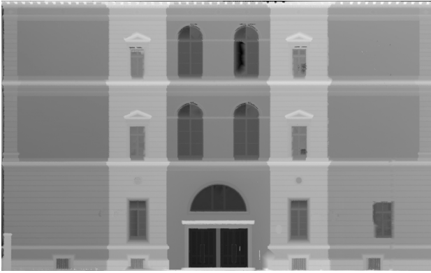
Figure 9. LASERMAP of a single facade derived from the point cloud.
