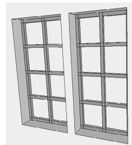
Figure 6. Reconstructed crossbars for two windows.
