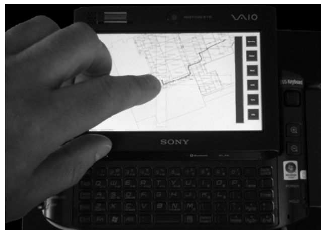
Fig. 1: Current prototype of the TANIA system. By tapping on its touch screen with tactile overlay information about the location and current environment can be received. Several soft keys and hardware keys control the system. Map operations such as scrolling and zooming can be done with cursor keys. The keyboard can be used to insert augmented text information about the current location and to search for objects and information.
