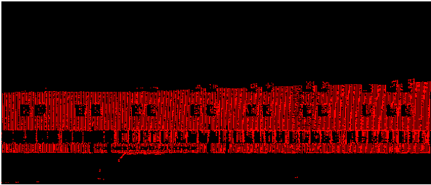
Figure 11: Points from right scanner (4), measured in epoch 2, at a mean range of approximately 15m.
