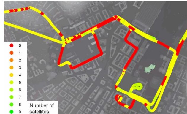
Figure 5 : Measured trajectory with number of visible satellites, overlaid to DSM of test area.
