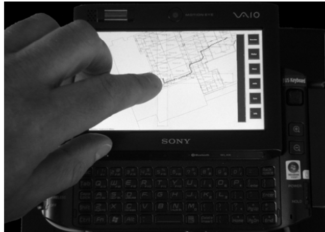
Figure 1: Prototype of the TANIA system. By tapping on the touch screen information about the location and current environment can be received. Map operations such as scrolling and zooming can be done with a joystick and a cursor. Several soft keys and hardware keys control the system. The keyboard can be used to insert augmented text information about the current location and to search for objects and information.
