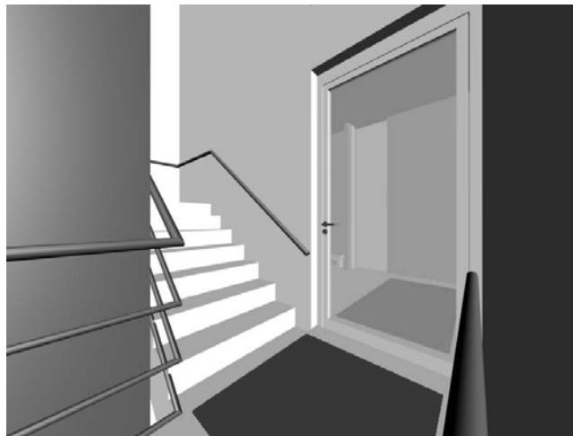
Figure 2: Virtual information areas (rectangles on the floor) can be inserted into 3D models or 2D maps in such places as hallway intersections or at stairways. Augmented information can be linked to these areas, via keyboard, by map makers or blind users.
