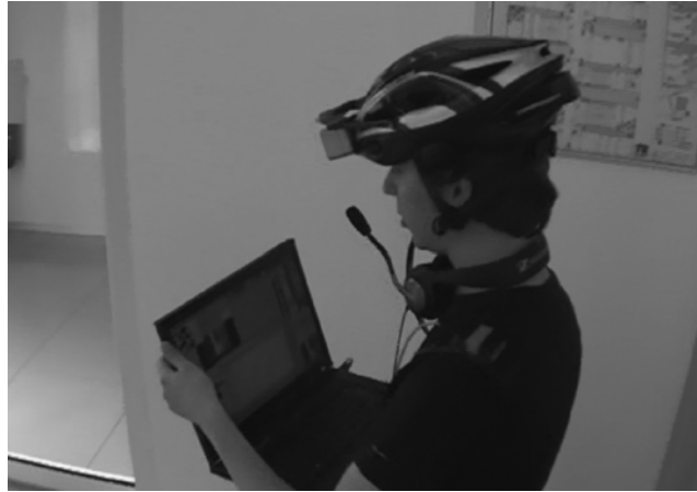
Figure 3: The navigation system and object recognition system is based on detailed 3D environment models. The complete system can be controlled via voice using a headset.
