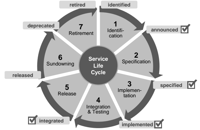
Fig. 1. Service Life Cycle with Service States and Checkpoints
