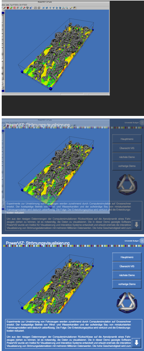
Figure 3: Clipping the user interface. Top: application after being started with the preload library (background color, position, and size are being set, UI partially clipped at desk-top); bottom: final result as seen by the user (UI clipped at window mask).
